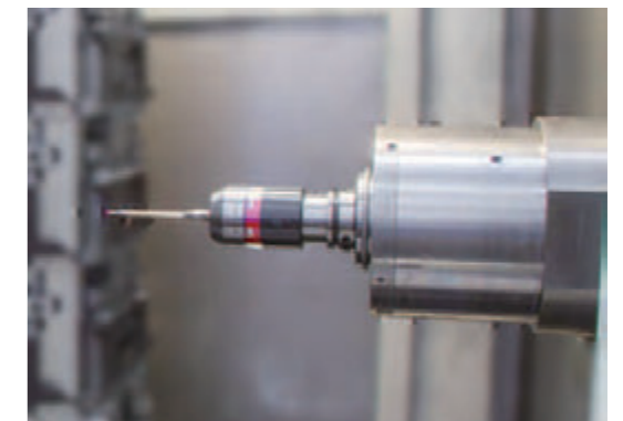
▲ Wireless workpiece measurement system, no cover issue
