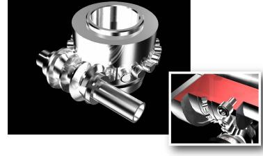
Cam type transmission device has the advantages of zero-backlash, accurate deceleration, and high rigidity. In addition, compare with the traditional worm gear and wheel, its high speed positioning is two times faster. Furthermore, it performs well in both heavy duty machining as well as complicated workpieces.
