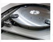
Pallets are driven by servo transmission devices. Each pallet allows 90 degrees rotation for facilitating the operator in loading and unloading workpieces and
