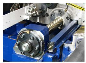
The preloaded ball screw reduces thermal distortion and ensures the machining performance and precision. Axis thirst bearings are auto lubricated.
