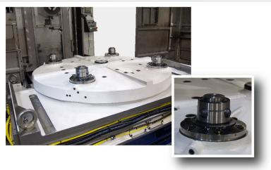
The full B axis utilizes a high pressure brake system for heavy cutting. Minimum positioning increment is 0.001 degrees.
