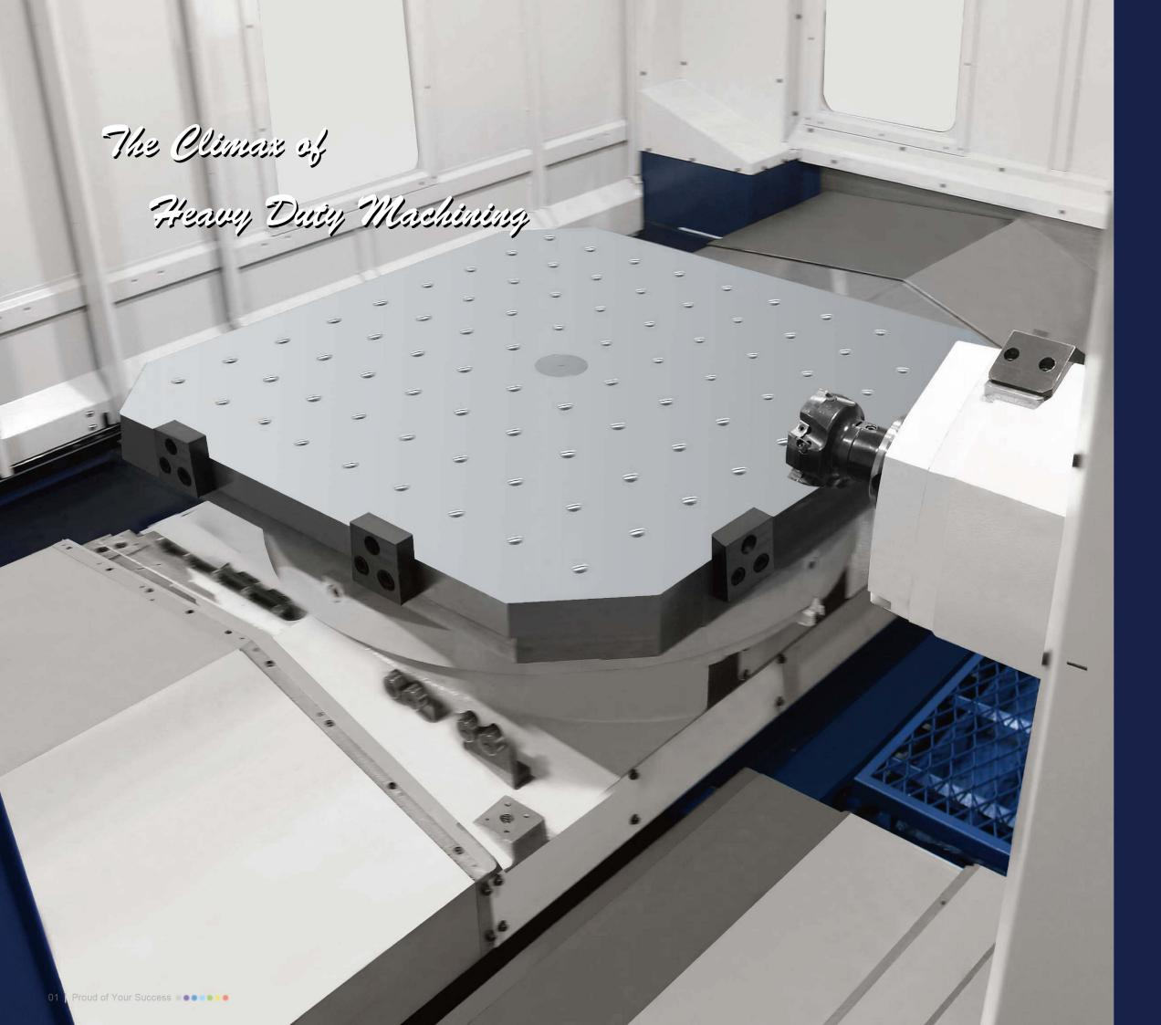
The HG-1250 is made from high-grade cast iron. It features hardened and ground box ways in all axes, providing high rigidity and excellent precision.
