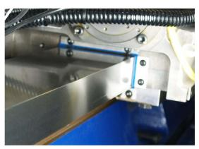
All three linear axes employ rigid box ways. The ways are induction hardened and then finely ground to satisfy both heavy cutting and high accuracy demands.
