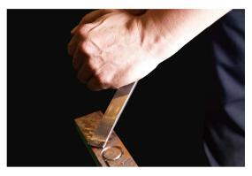
High precision scraping is carried out by skillful engineers to obtain the perfect lubrication with correct oil-film. The machine accuracy and the lifetime of slides are both raised accordingly.
