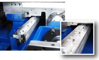
X/Y/Z axis adopts Heidenhain linear scale system for assuring the machining accuracy.
