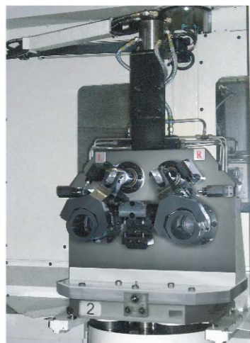
1. Suspended arm type supply Totally 6 ports are provided on each side and the maximum hydraulic pressure allowed is 250 bar.
